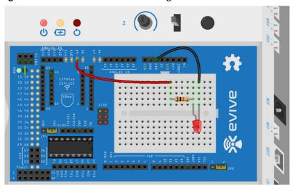
2. Controlling the state of the LED: Make the following circuit on evive Breadboard:
