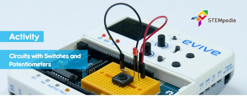
In this activity, you will learn how to control the brightness of a LED using potentiometer and state of the LED using switch.
