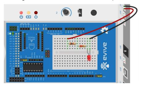
2. Parallel: Make the following circuit on evive Breadboard for parallel resistors (Use two 220 Ohm resistors):
