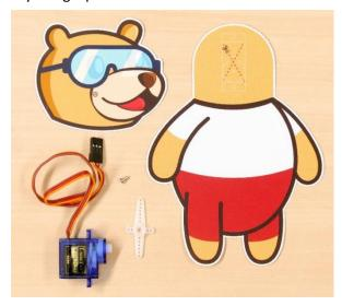
**2.** On the cutout of Tobi's body, there is a space marked for the servo motor. Cut and fold the flaps inwards to make support for the servo motor.
