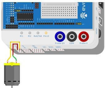
6. Power ON evive. A menu will open. If not, centre press on navigation key to bring the menu. Navigate to Controls > Motors > Motor 1.
