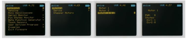
7. Control the speed using potentiometer and direction using slide switch.
