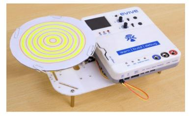
5. Insert the motor wires in the first motor channel, i.e. M1.
