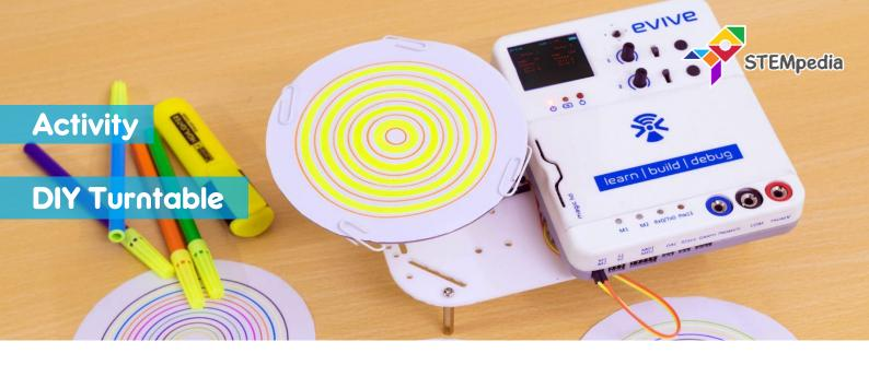
In this activity, you will learn how to make a small DIY turntable, whose speed and direction can be controlled using evive's slide switch and potentiometer.
