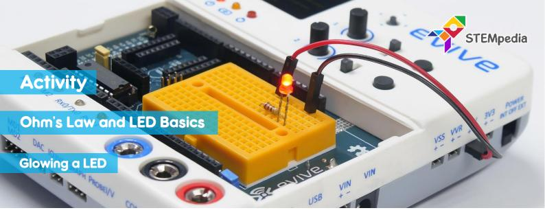
In this activity, you will learn how to glow a LED? You will also learn how the brightness of the LED changes when the value of the resistor is changes.
