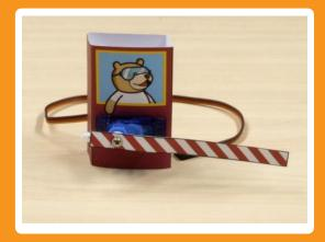
In this Activity, First We will construct a DIY Tollbooth and then make it open and close whenever we press tactile switch by programming it inside the PictoBlox.
