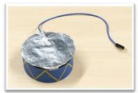
STEP 4: Connect one end of the jumper wires to the drum and gentle press the aluminum foil so that it remains in contact with its end point.
