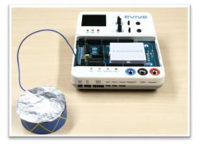
STEP 5: Connect other end of the jumper to evive's touch sensor 1.
